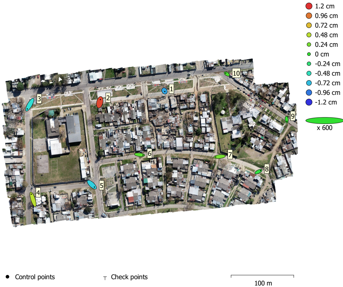
Fig. 4. GCP locations and error estimates.
